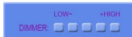
2. Press the [+] or [-] key for desired illumination of the control panel. Pressing DIM key also changes the illumination level.
