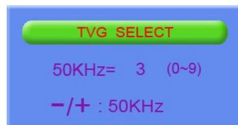
2. Set the TVG curve with [+] or [-]. The default level is 5. Attenuation compensation curve is at 20LogR curve.
