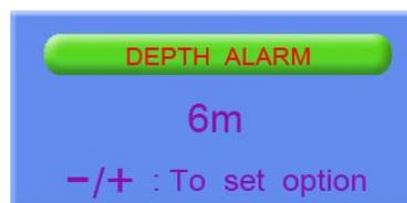
2. Press the [+] or [-] key to change setting depth. The setting is shown digitally at the top of the screen and graphically key the depth alarm line.
