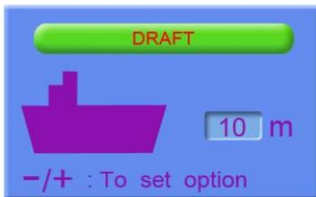
3. Press the [+] key to increase the setting depth and [-] key to decrease it. The setting depth is -10 to 30 m in steps of 0.1 m.
