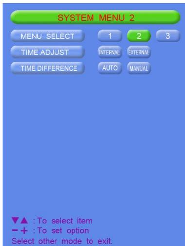
**TIME DIFFERENCE:** Selects auto (UTC) or manual. Auto uses the time difference in ZDA (IEC 61162-1). In manual, it is necessary to enter the time difference in hours and minutes.
